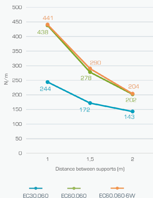
Safe working loads 60mm width basket trays
